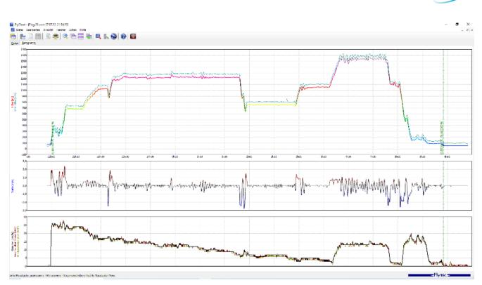
Complete documentation of the 8-hour course in the Flytec 6040: Note the stable altitude accuracy of 6-8 m standard deviation over hours, which can never be achieved by hand! The intermittent variations resulted from the bottle change and the subsequent manual burner tests. This allows the burning time of the individual cylinders to be easily assigned and verified.
